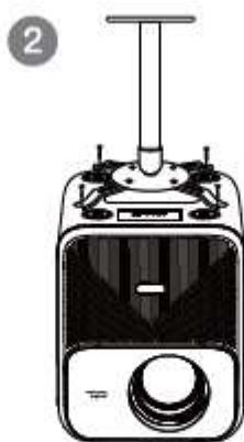
Adjust hanger angle to align with the hole and then tighten screws (4 pcs of UNC 1/4"-20 × 3/8 )
